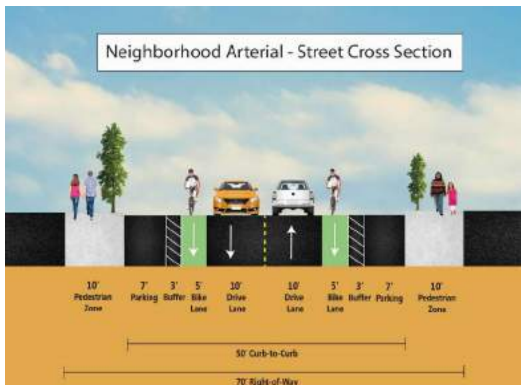
Figure 25: Street Cross Section Example: Neighborhood Arterial
