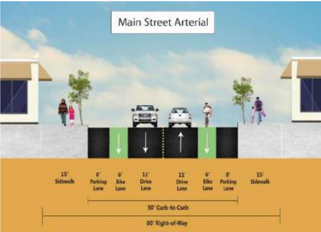
Figure 23: Street Cross Section Example: Main Street Arterial
