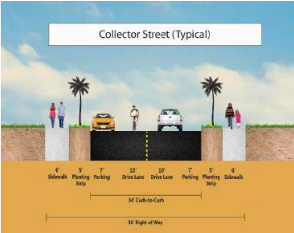
Figure 26: Street Cross Section Example: Collector Street
